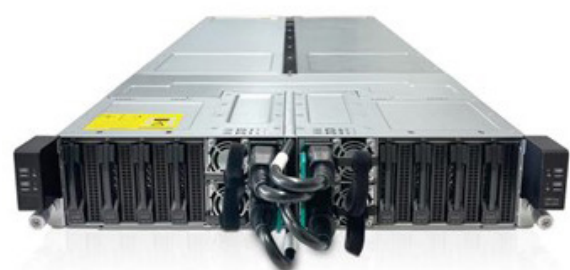
Figure 4. Density-optimized HPE Cray XD2000 chassis supporting up to 4x HPE Cray XD225v 1U servers or 2x HPE Cray XD295v 2U servers
