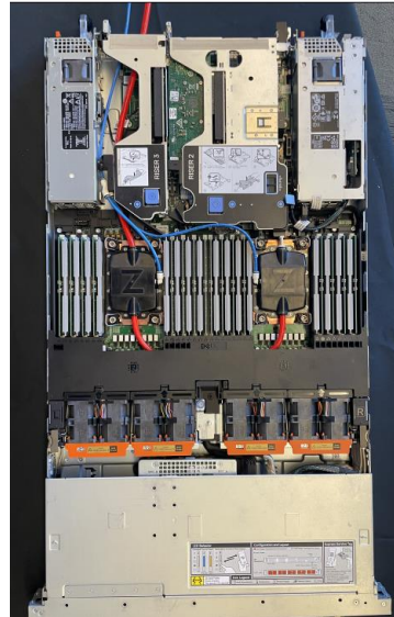
Figure 8: Waterless On-Chip-Coolong (Source: ZutaCore)
